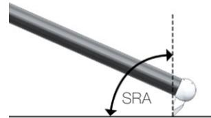
The Stylus Rake Angle (SRA - see figure) is very important to the performance of the Replicant 100 stylus, and the long contact surface (the sharp edge) of the diamond should be almost perpendicular to the record surface when viewed from the side. The angle between the record surface and the cantilever is close to 23 degrees when SRA is 90 degrees.
