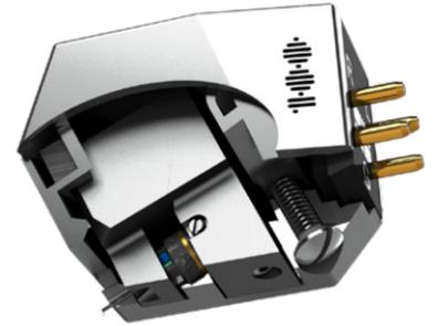
The use of this optimized magnet system allows for the use of a lightweight, non-magnetic armature, which also provides noteworthy benefit to the dynamic capability of the MC Century. The reason for this is that our high-tech polymer-based armature has almost no influence on the magnetic field during movement. Hence when combined with ultrapure oxygen-free copper coil wire, it delivers perfect reproduction of the cantilever movements without compromise.
